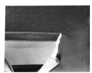
Mark the position of the cover strip on the no. 3 crossmember and ease the strip off.
