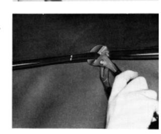
Press the headlining onto the doublesided adhesive tape on the no. 4 crossmember and screw the metal strip into position. Note that the strap for the rear screen is retained by means of the middle screw.
