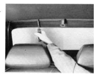
4 Pull away the headlining from the adhesive tape holding it in place on the no. 4 crossmember and let it hang free.
