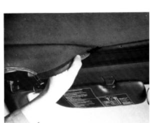
Lift the headlining into position and press was removed.
