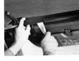
9 Pull the headlining away from the adhesive tape holding it in position on the no. 1 crossmember and lift it out of the car.
