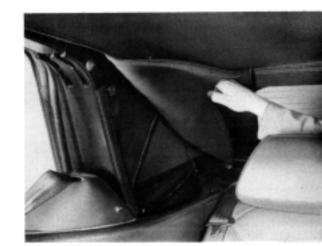
2 Undo the zip, release the strap and lower the rear screen.
