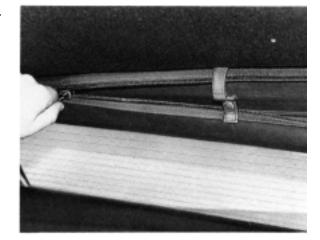
3 Undo the retaining screws and remove the strip from the no. 4 top-assembly crossmember.
