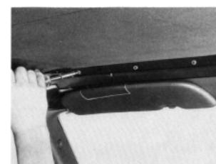
Press the plastic retainer strip into position on the no. 3 crossmember. Ensure the strip is positioned centrally by lining up the marks made before the strip was removed.
