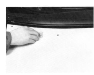
2 Remove all traces of old adhesive and dirt from the spoiler assembly.
