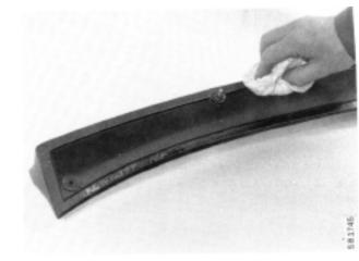
3 Fit double-sided adhesive tape, part no. 78 74 662, along the spoiler.
