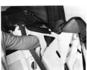
6 Remove the wing nut from the rear fastening (access through the flap in the trim inside the luggage compartment).
