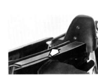
Remove the wing nut from the rear fastening (access through the flap in the trim inside the luggage compartment).
