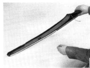
4 Make sure that the rubber washers and cable at the rear fastening are in place.
