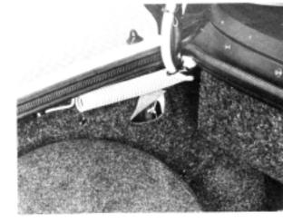
3 Use a heat gun to release the tape. Take care not to apply too much heat as this can damage the paintwork or spoiler assembly.
