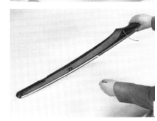
4 Make sure that the rubber washers and cable at the rear fastening are in place.
