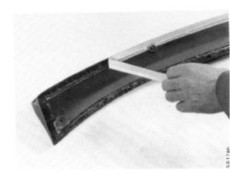
4 Apply Sikaflex 255 around the hole for the wiring to the stoplight.
