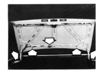
3 Use a heat gun to allow the tape to be pulled away. Take care not to apply too much heat as this can damage the paintwork or spoiler assembly.
