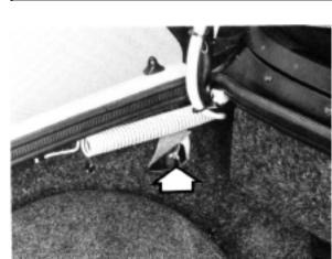
6 Fit and tighten the nut on the middle stud.
