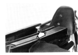
5 Open the top halfway and remove the nut from the middle stud.
