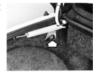
7 Use a heat gun to release the tape. Take care not to apply too much heat as this can damage the paintwork or spoiler assembly.
