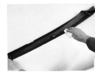
3 Fit double-sided adhesive tape, part no. 78 74 662, along the spoiler.
