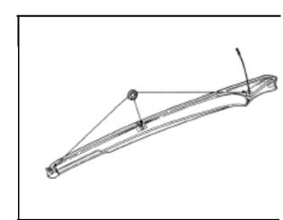
5 Position the spoiler assembly on the car and screw down tight the wing nut on the rear stud.
