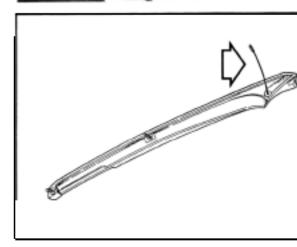
9 Save the cable in the rear mounting hole as this will be needed in the fitting of a new spoiler assembly (where applicable).
