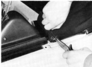
82 92492 or 8 Fit the spacers, part no. 82 92 799, as appropriate, into position on the windscreen frame.
