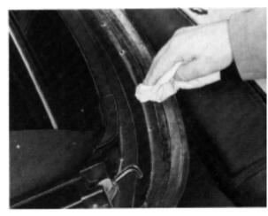
2 Remove all traces of dirt and old adhesive from the underside of the no. 1 Cross-member.
