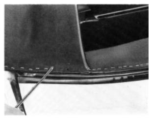
24 Undo the screws securing the anti-ballooning strips to the no. 2 and no. 3 **Cross**members (the strips are in the pockets in the top cover).
