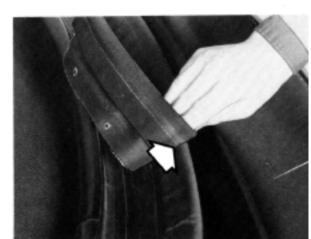
23 Open up the bottom flap of the welt cord and staple it to the plastic strip, starting in the middle and working out towards the ends. Use the long staples, part no. 69 34 285.
