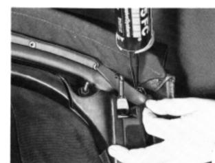
31 Place the spacers, part no. 82 92492 or 82 92 799, as appropriate, in the wind-screen frame. Raise the top and engage the latching hooks but do not close the latching handles.
