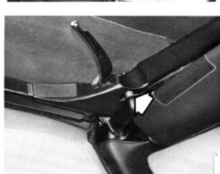
32 Stretch the top fabric by pulling it down over the rails at the back and glue the top to the rails.
