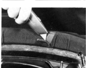
20 Cut through any creases along the length and smooth the fabric down.
