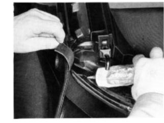
17 Glue the top cover to the no. 1 Cross-member. Fold the fabric carefully over the crossmember to ensure a mini- mum of creasing.
