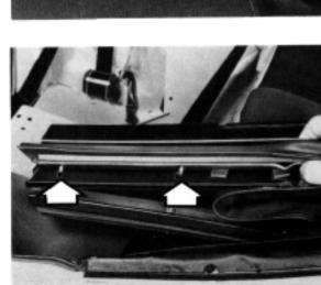
28 Fit the screws securing the seal to the no. 1 crossmember.
