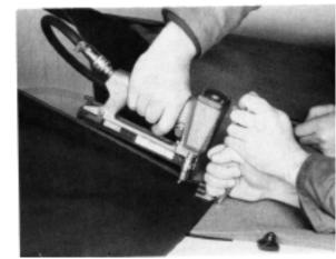
43 Pull down the top cover side flaps to stretch them and staple the front part of the side flaps in position. Do not staple in the holes in the stretcher.
