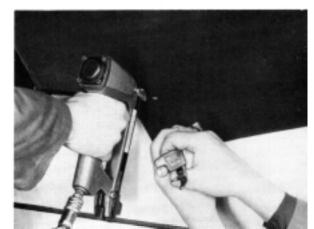
**39** Remove the staples in the side panels, stretch the fabric again and use a couple of staples to hold it in place.
