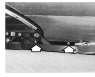
55 Fit the screws securing the anti-ballooning strips inside the pockets on the no. 2 and no. 3 crossmembers.
