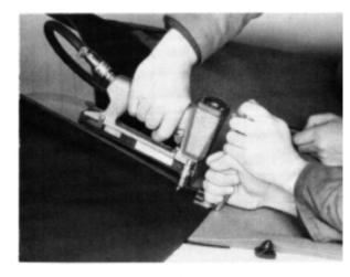
36 Stretch the top cover by pulling it down and towards the rear of the car at the side, and secure with a couple of staples.
