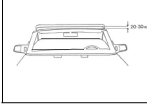
Check the adjustment of the latching hooks by latching the top in position and then pressing down on the front corners of the top. No play should be present.
