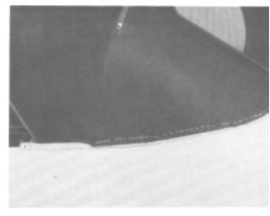
54 Adjust the position of the front seal snug against the door glass and tighten the nuts securing the seal retainer.
