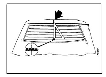
2 Mark the midway position along the no. 4 crossmember. This should be in line with the retaining screw for the strap.
