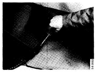
31 Remove the spacers from the windscreen frame and raise the top assembly.
