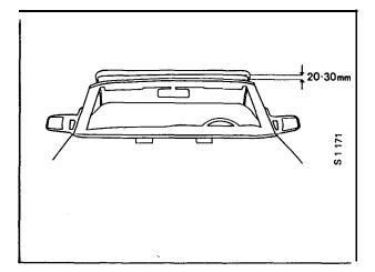
Check the adjustment of the latching hooks by latching the top in position and then pressing down on the front corners of the top. No play should be present.
