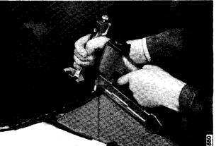
17 Stretch the top cover on either side by pulling it down and towards the rear, and secure by means of a couple of staples.
