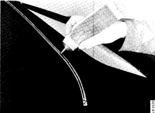
29 Press the feature strip into position and screw on the end caps.
