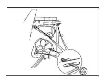
4 Undo the nut securing the glass to the glass-lift mechanism and turn the stud in the appropriate direction.
