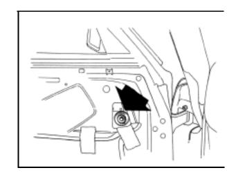
2 To adjust the height of the rear end of the glass, loosen the screw in the rear glass stop.
