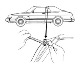
On being raised, the leading edge of the top should stop in the park position, 20 = 30 mm (0.79 - 1.18 in) above the wind-screen frame. The front of the top must also be parallel with the frame.
