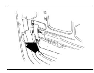
3 The height of the trailing end of the door can also be adjusted by undoing the rear nut on the window glass lift mechanism.
