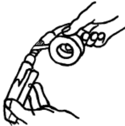
Figure 7. Wrapping Insulating Tape on leads
