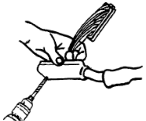
Figure 5. Drilling 7mm drainage hole
